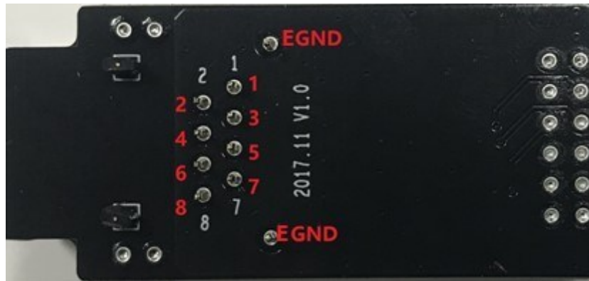
Figure 4. Eport Pro-EP20-PIN Pins Map
