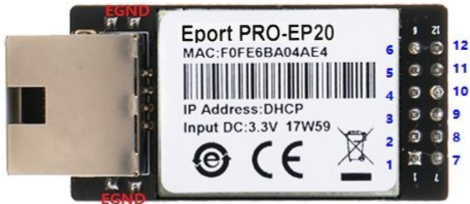
Figure 3. Eport Pro-EP20 Series Pins Map
